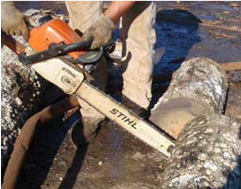
Figure 4. Cutting Lower Portion of Copper Dock Pile for Test Sections
