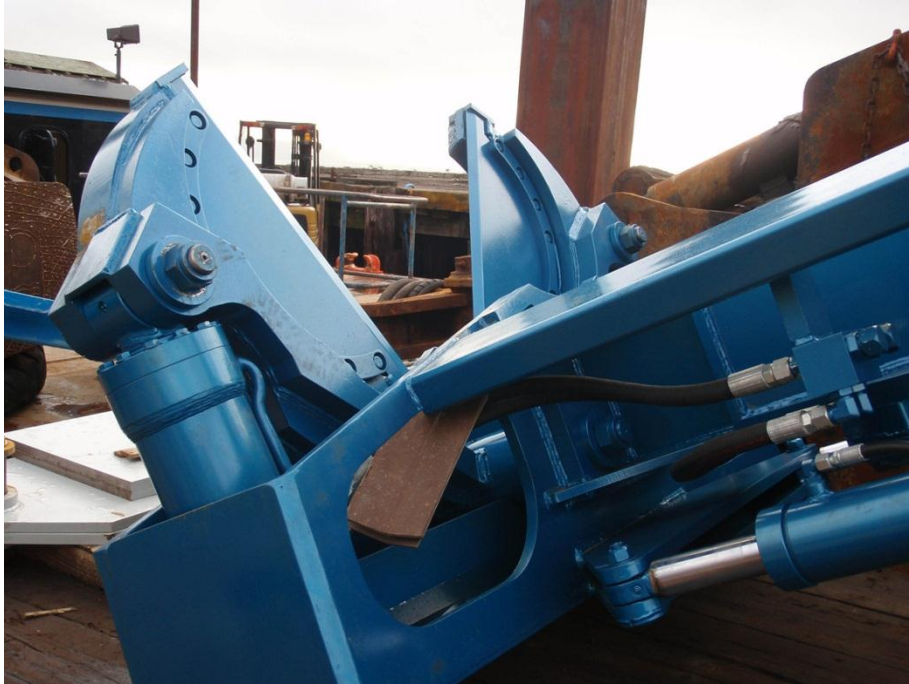
Figure 2. Shear Used to Cut ASARCO Docks Piles
